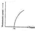
Collector at suitable +ve potential Intensity constant Frequency increased No emission till certain frequency vo vo is characteristic of the material of emitter plate vo called threshold frequency v>=vo, emission takes place \( \lambda \) called threshold wavelength
