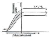
For a given curve: v constant(v>vo) & intensity constant +ve potential at collector increased, current increases
