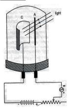
Works on the principle of photoelectric effect Construction: It consists of a semicylindrical photosensitive metal plate C (emitter) and a wire loop A, (collector) supported in an evacuated glass bulb. It is connected to a high tension battery and a microammeter. Working: When light of suitable wavelength falls on the emitter. photoelectrons are emitted. These are attracted by the collector. A small current flows through the circuit. which is recorded by the microammeter. If the intensity Is
