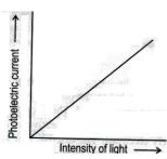
Collector at suitable +ve potential Frequency constant and above vo Intensity of light varied Current increases linearly with increase in Intensity Number of photoelectrons emitted per second is directly proportional to the intensity of incident
